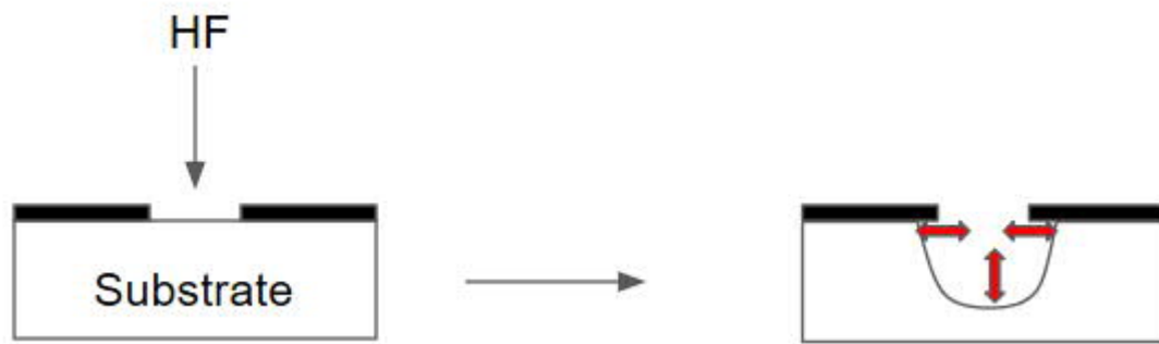
Figure 2: Etching profile of isotropic etching, etchant works towards all directions, creating an inhomogeneous semi-circular feature. Red arrows represent the same amount distance coverage of the etching procedure. Sum of the underetching distance is approximately, double the value of depth distance. Thicker black lines represent protective mask.
