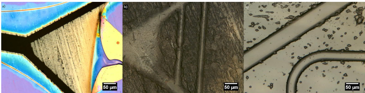
Figure 14: Effect of 48% HF on pure chromium layers. Unnecessary exposure to Nichrome etchant lifted-off the chromium layer (a). Etching the damaged sample for 30 seconds resulted in eroded surface and cracked channels (b). Etching of the undamaged sample for 40 seconds, chromium mask provided enough protection for etched channels; however, surface was still exposed to damage. All three images contain 50 \mu\text{m} scale bars.
