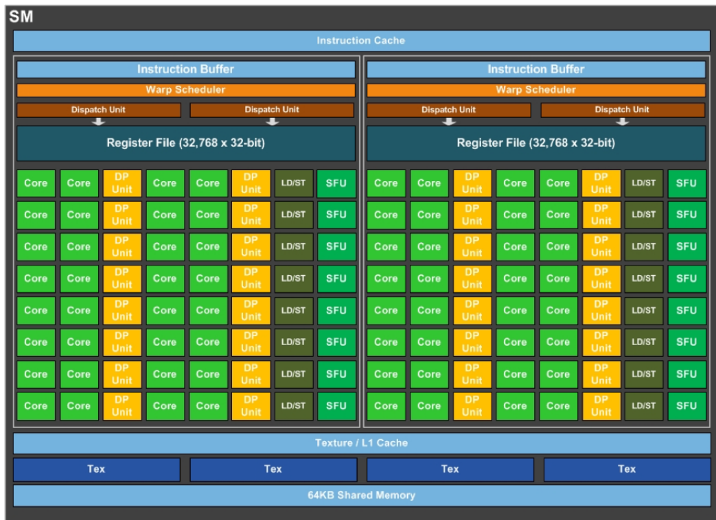
Figure 6. A block diagram of a single Streaming Multiprocessor (NVIDIA 2016b)).
