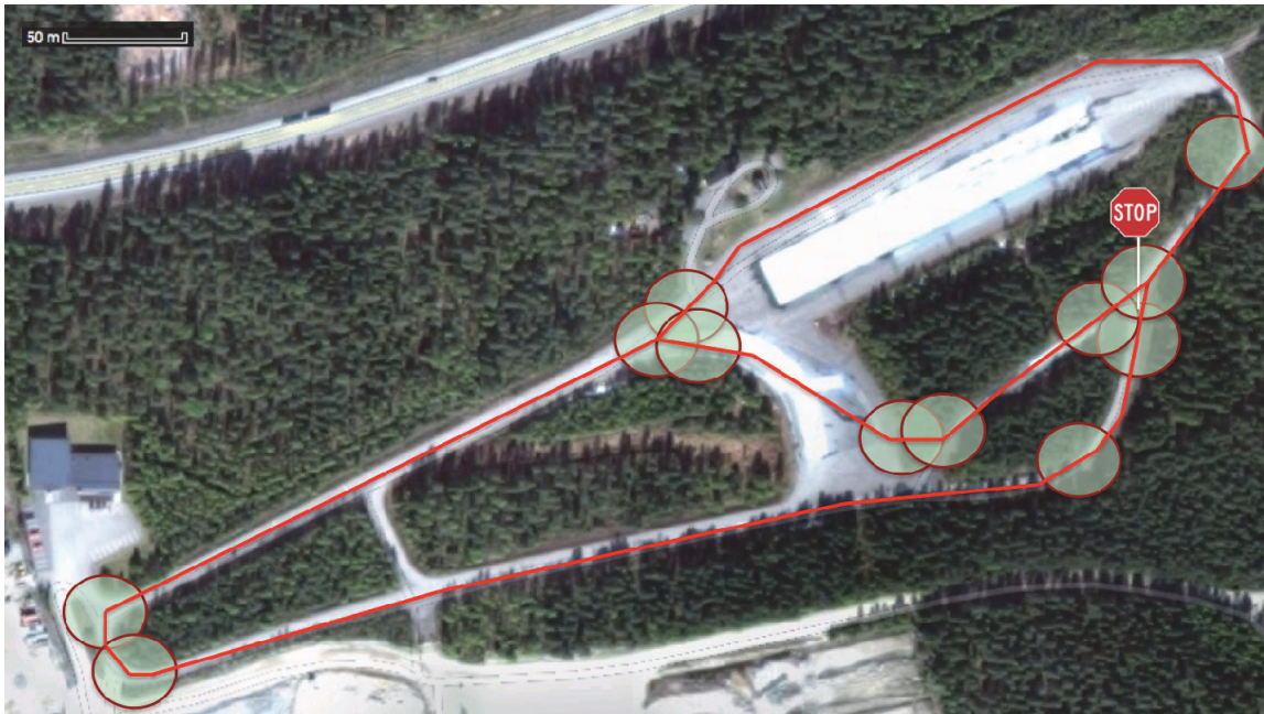
Figure 5. The driving paths on the track. The circles indicate high demand areas with WT=0 , the intersection marked with stop a sign being the most demanding area.
