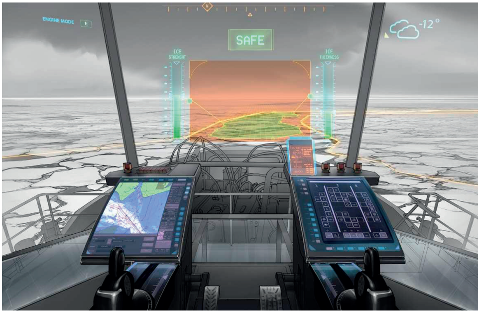
Figure 4. The Sea-Ice Analyser concept – the ship bridge presents information on ice thickness and strength and indicates whether or not it is safe to proceed. (© 2013 Rolls-Royce plc)
