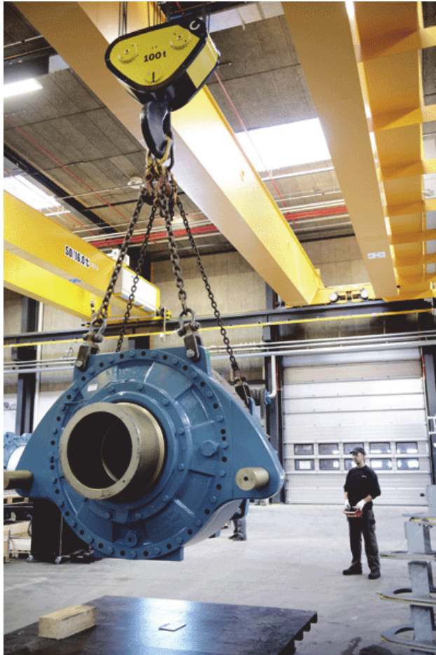
Figure 2. Operating an EOT crane in a factory.
