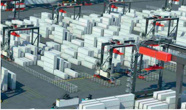
Figure 1. A visualization of remotely operated container cranes in the truck loading zone. The smaller cranes in the top part of the figure are ASCs.
