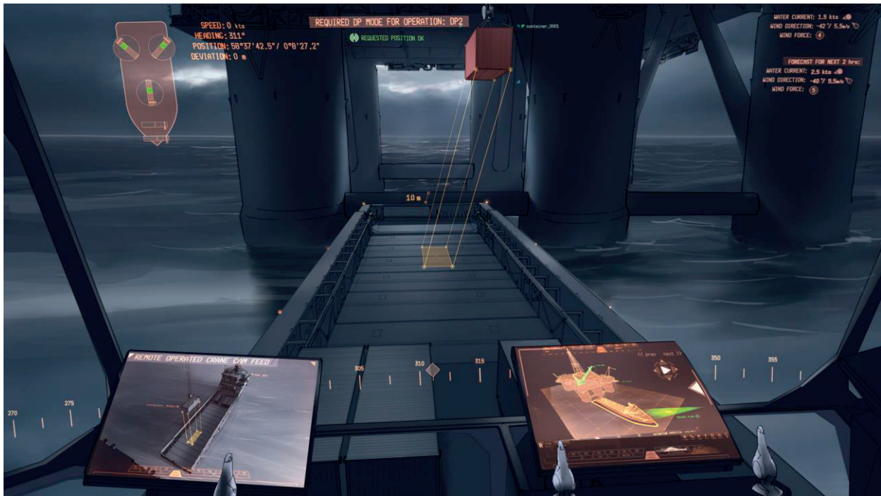
Figure 2. The Augmented Crane Operations Concept (© 2013 Rolls-Royce plc).
