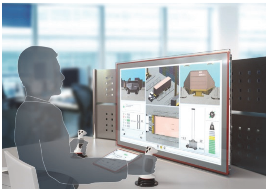
FIGURE 7 Concept illustration of the ROS system with the four-view setup in the main display (from Article VIII) © Konecranes
