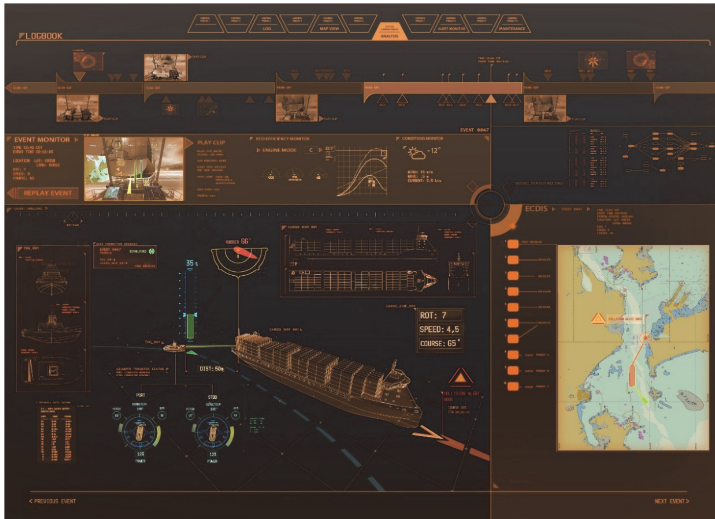
FIGURE 9 A user interface concept illustration of the 'Logbook' system for tugboats from the FSB case © Rolls-Royce
