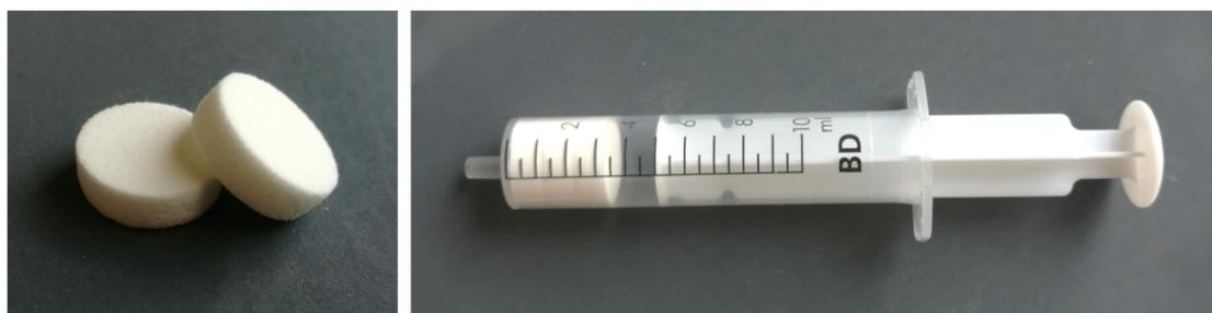
FIGURE 24 Image of the PP-21K filters (left) and of the 10 mL syringe with three PP-21K filters that was used for the adsorption experiments (right).
