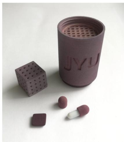
FIGURE 31 Image of different SLS 3D printed PA12 objects that have been functionalized with gold.
