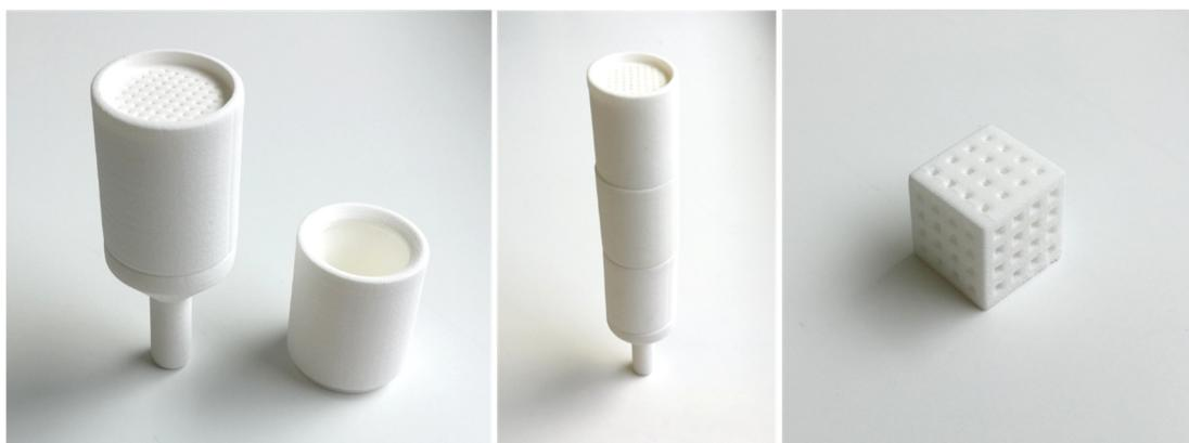
**FIGURE 23** Image of the SLS 3D printed PA12 filter objects with one (left) and three (middle) filter units attached. Image of the SLS 3D printed PA12 mesh cube (right).
