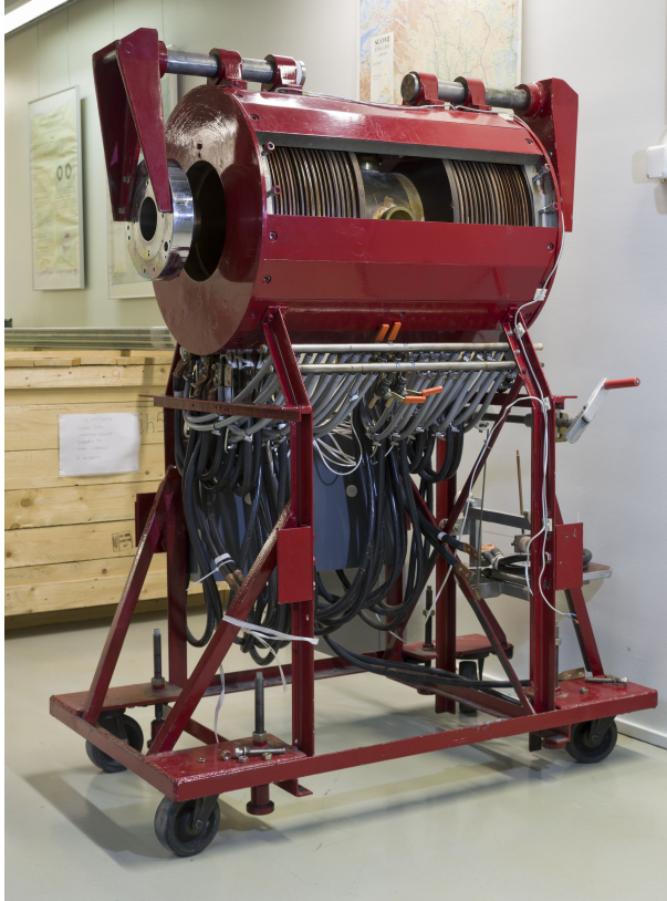
Figure 2. On left is the spectrometer that is used for guiding the electrons [7]. On right is a source holder used during the test measurements with different sources.
