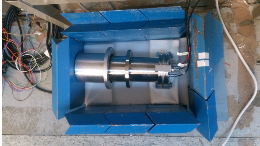
Figure 8. Scionix detector was protected with a Germanium detector -cup inside the lead cave.
