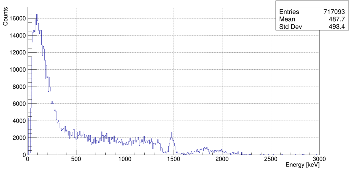
Figure 11. A figure of a background measurement made with LaBr 3 detector.
