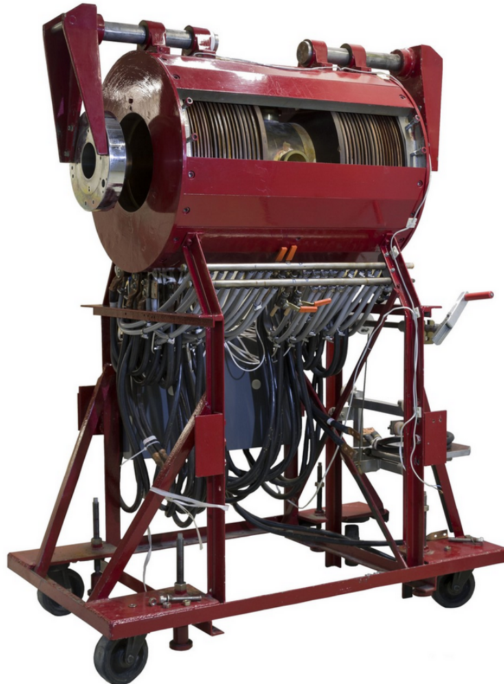
Figure 10. The Siegbahn-Slätis type intermediate-image spectrometer used for the experiment. From the side two iron covers have been removed to reveal the current carrying coils.
