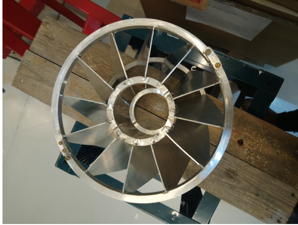
Figure 14. The positron baffle used around the shield. The electrons bend due to the magnetic field to the direction where they go between the Al plates when positrons bend to the other way hitting and stopping into the Al plates.
