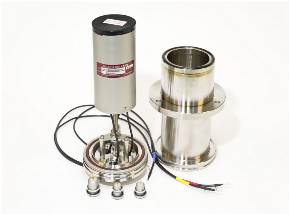
Figure 17. The Scionix detector mounted on its holder and a black cover covering the entrance window from light.
