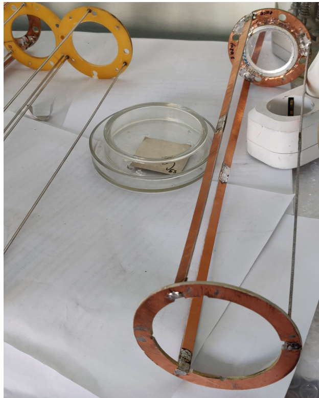
Figure 22. 59 Co and Si targets. Silicon target is mounted on the target holder.
