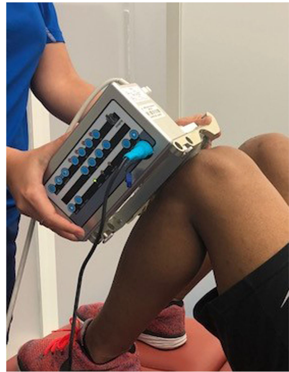
Fig. 2 Lateral view of UTC tracking device showing silicone pad in contact with left patellar tendon
