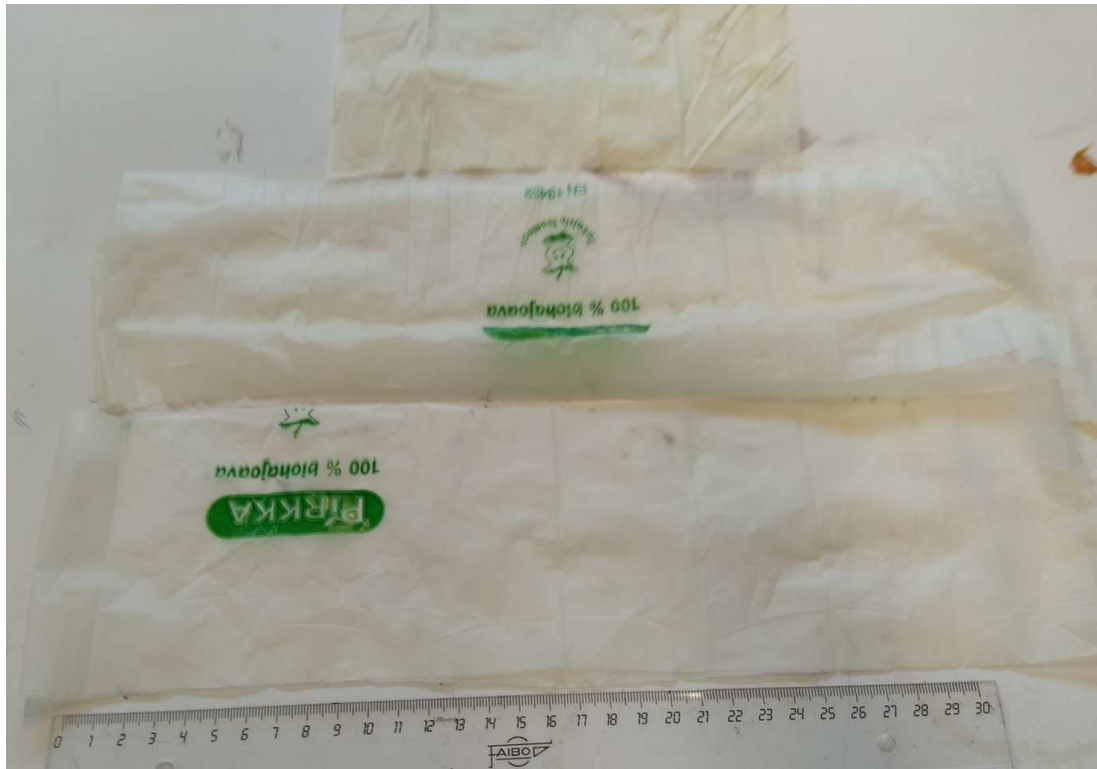
Figure 2. Example of pieces of a bioplastic bag pieces added to a reactor
