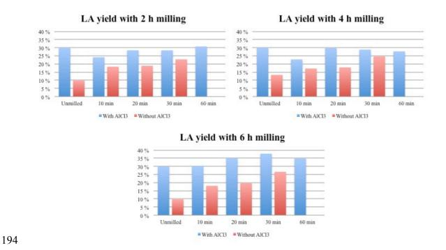
Figure 1. The effect of the milling time and the conditions of the subsequent conversion reaction on the LA yield. Conversion reaction temperature (180 °C) and the amount AlCl<sub>3</sub> catalyst (5 mg, when used) were kept constant. The conversion reaction time for the unmilled pine sawdust was 60 min.
