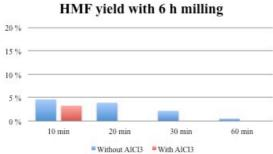
Figure 4. The effect of the milling time and the conditions of the subsequent conversion reaction on the HMF yield. Conversion reaction temperature (180 °C) and the amount AlCl<sub>3</sub> catalyst (5 mg, when used) were kept constant.
