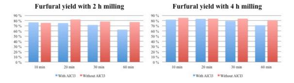
Figure 2. The effect of the milling time and the conditions of the subsequent conversion reaction on the furfural yield. Conversion reaction temperature (180 °C) and the amount AlCl<sub>3</sub> catalyst (5 mg, when used) were kept constant.
