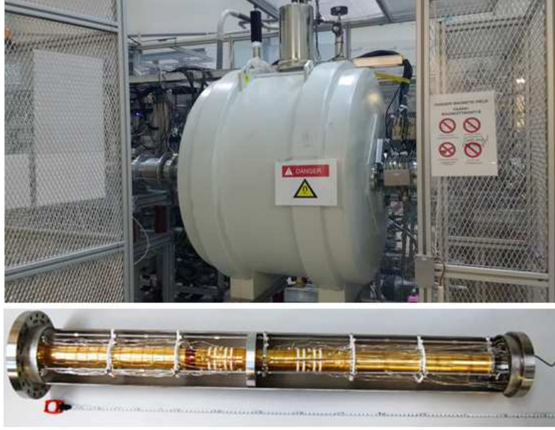
FIGURE 17 The 7 T superconducting magnet housing the JYFLTRAP Penning trap (top) and the JYFLTRAP with its different electrodes (bottom).
