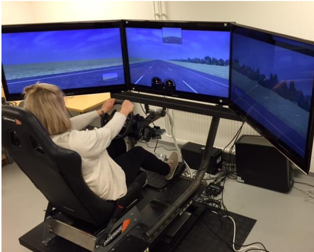
Figure 1: The driving simulator on a 2-DOF motion platform and the driving environment.
