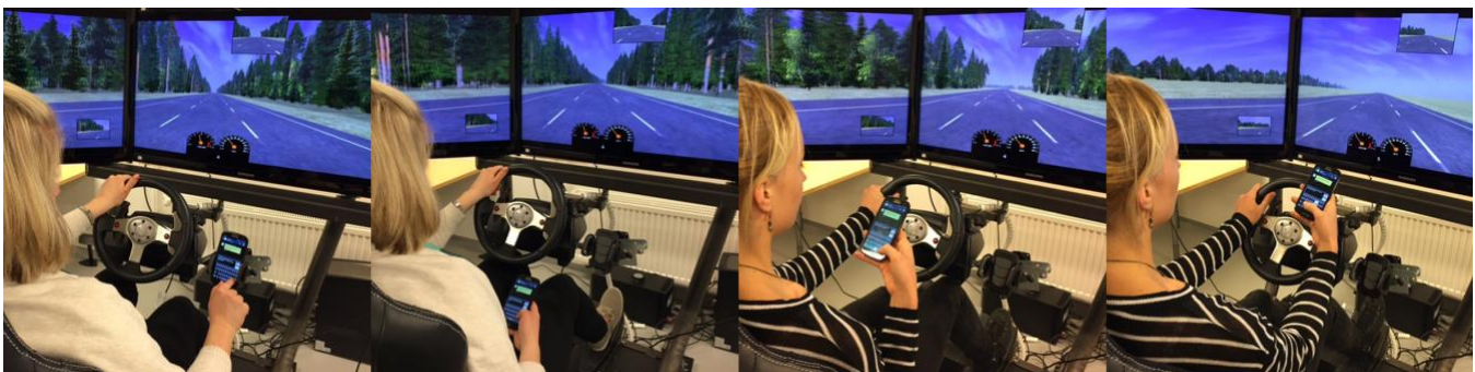
Figure 2: Texting the phone on the holder versus the most popular hand-held texting styles. From left: phone on the holder, phone on the lap, phone in between the participant and the steering wheel, and phone close to the steering wheel.
