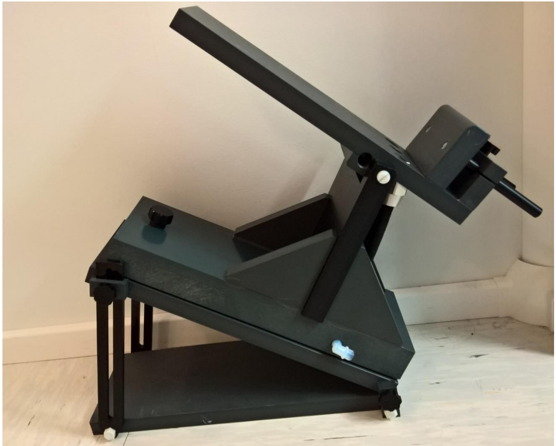
FIGURE 5. Adjustable pneumatic ankle movement actuator used in the study.
