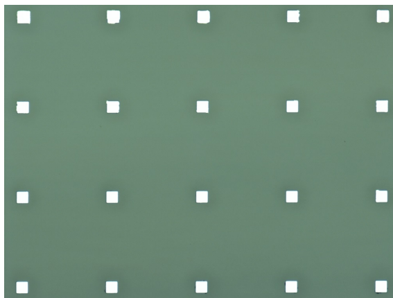
Figure 10. Optical micrograph of the chromium mask for photoresist patterning. Light areas are metal, dark areas are glass. One row is left out from the picture. Size of the squares is 50\ \mu\text{m} \times 50\ \mu\text{m} .
