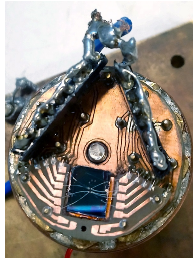
(b) Bonded sample. Grounding is still attached to sample stage.
