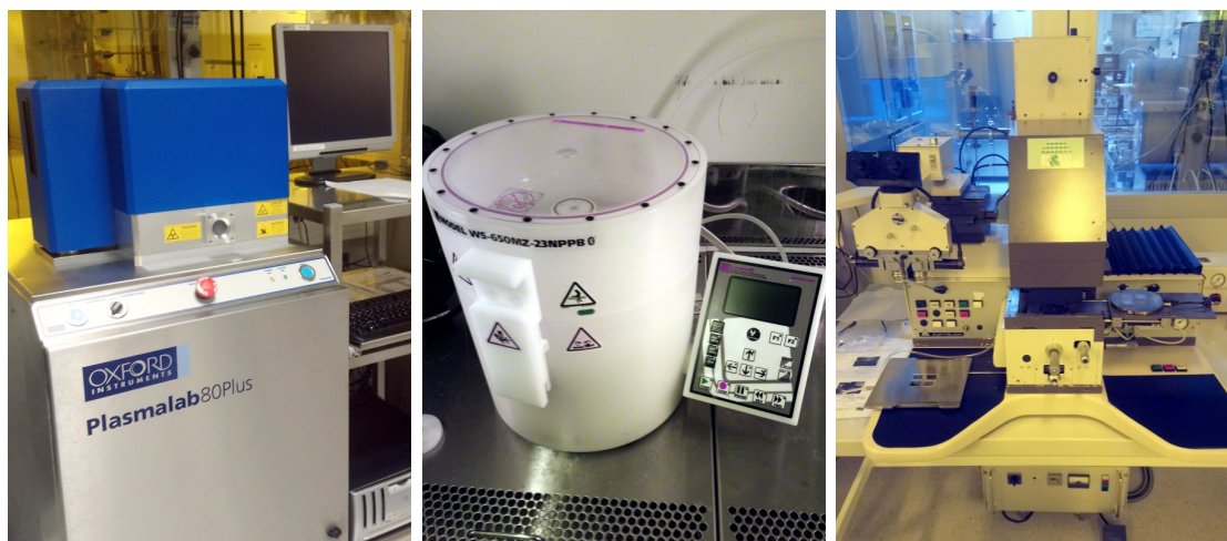
(a) RIE Oxford instruments Plasmalab80Plus. (b) Laurell Model WS-650MZ-23NPPB spin coater. (c) Karl-Suss MA45 UV mask aligner.
