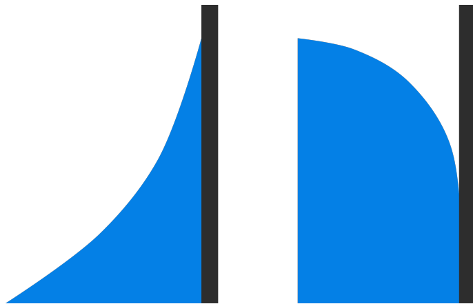
Figure 7. Shape of the meniscus when water is in contact with hydrophilic surface (left) and hydrophobic surface (right).
