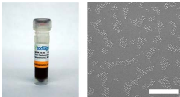
FIGURE 7.1 (a) 5 nm biotin gold nanoparticles from Cytodiagnosics; (b) SEM image of b-AuNPs on silicon oxide with RIE treatment. Scale bar of 200 nm
