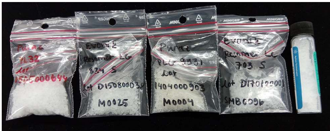
Figure 17. Used materials. From the left, PLLA (inherent viscosity 3.2 dl/g), PLGA (produced by Evonik, inherent viscosity of 2.2 dl/g), PLGA (produced by Purac, inherent viscosity of 3.11 dl/g), PLCL (inherent viscosity of 1.5 dl/g), and polystyrene standard ( M_p = 70500 g/mol).
