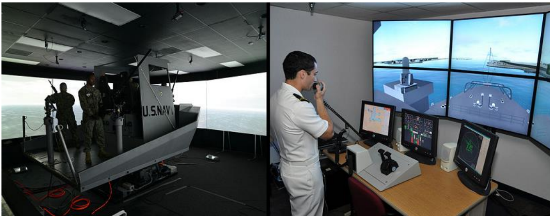
FIGURE 2 Left a ship simulator with a motion platform to improve behavioural realism. Right a ship bridge and multi-display vision system to improve physical realism of the simulator. (Wikimedia Commons US Navy)
