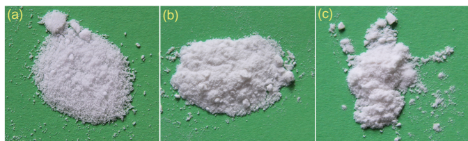
Figure 6: Precipitated struvite precipitates from (a) synthetic solution (Struvite:C) and (b-c) batch 1-2 (Struvite:B1-B2).
