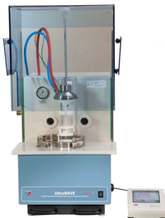
Figure 5: A single reaction chamber microwave assisted digestion system UltraWAVE equipped with control unit (right), manufactured by Milestone Srl. Samples in test tubes made of regular or quartz glass equipped with pressure balancing caps are placed inside pressurised PTFE container. 35
