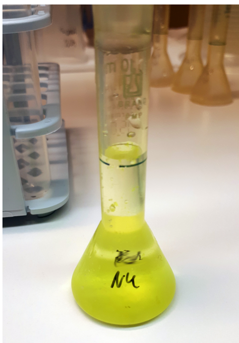
Figure 20: Digested sample transferred in volumetric flask, undigested yellow residue can be seen in the bottom
