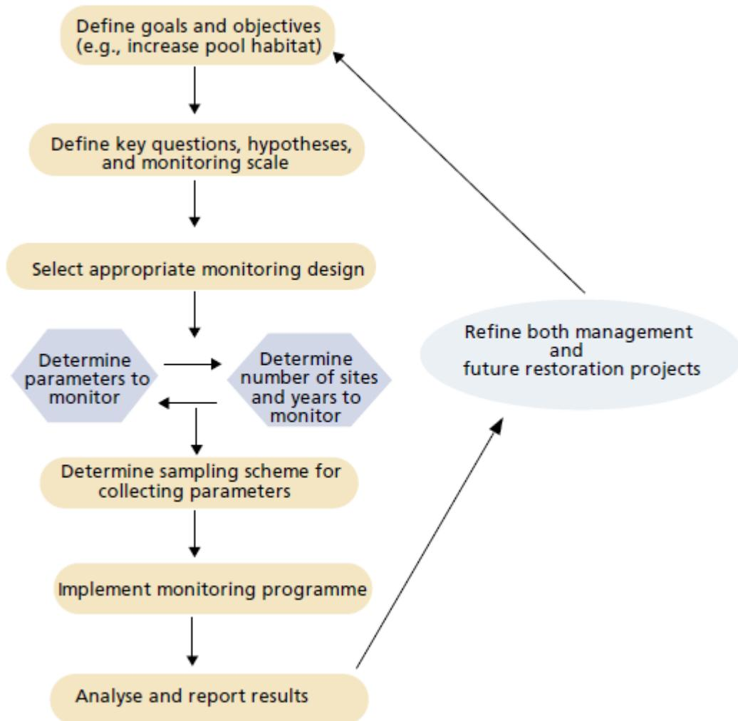
Figure 2. Key steps in developing a comprehensive monitoring program for restoration measures (Roni et al. 2005).
