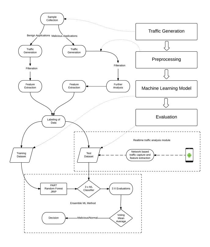
Fig. 1: Ensemble Machine Learning model for Intrusion Detection
