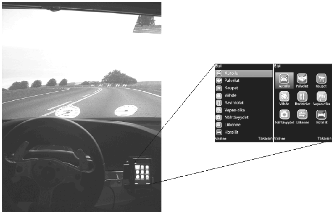
Figure 1. Driving scene from a participant's point of view indicating a leftward lane drift and the two alternative menu structures of the navigation software, List and Grid .
