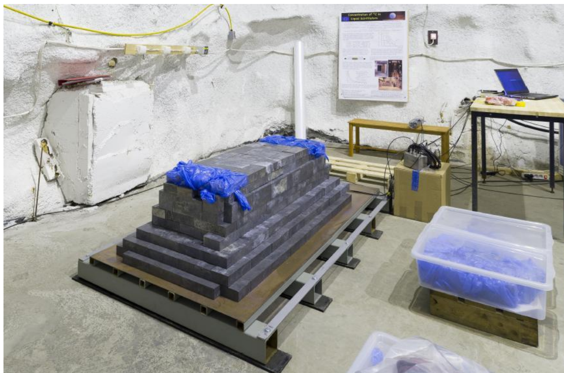
Figure 5. Shielding of the set-up for measurements of ^{14}\text{C} concentration.
