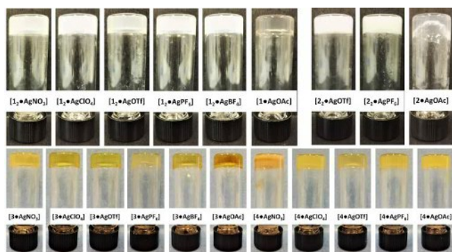
Figure 3. Photographs of gels prepared from ligands 1-4 with various silver salts in aqueous DMSO.
