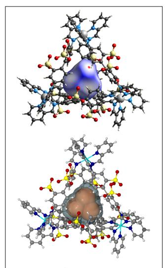
**Figure 4.** The Hirshfeld<sup>24</sup> surface plot (top) of the P<sub>4</sub> guest in the cavity of the metallocage.<sup>64</sup> The ball&stick view of the COSZOA<sup>1</sup> structure (bottom), the encapsulated guest with CPK style and the cavity volume surface<sup>26-28</sup> (1.2 Å probe) in transparent grey. Counter cations and solvent molecules are excluded for clarity.
