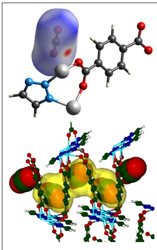
**Figure 10.** The Hirshfeld<sup>24</sup> surface plot (top) of the CO<sub>2</sub> guest in the pores of the Zn(II)-MOF (only asymmetric unit is shown). The ball&stick view of the DAFSEL<sup>1</sup> structure (bottom), the encapsulated guest with CPK style and the cavity volume surface<sup>26-28</sup> (1.20 Å probe) in transparent yellow.
