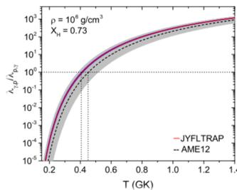
**Fig. 1.** Ratio of the photodisintegration to the proton-capture rates for typical XRB conditions. The uncertainties related to the JYFLTRAP  $Q$  value are shown by the blue lines and to the AME12 value by the gray-shaded area.
