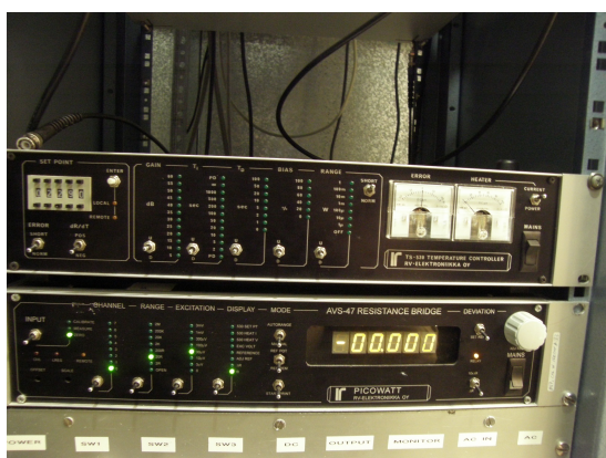
Figure 26. Above the TS-530 Temperature controller and below the AVS-47 resistance bridge.
