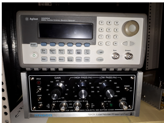
Figure 24. Above Agilent 33250A function generator and below Ithaco 1201 low noise pre amplifier.
