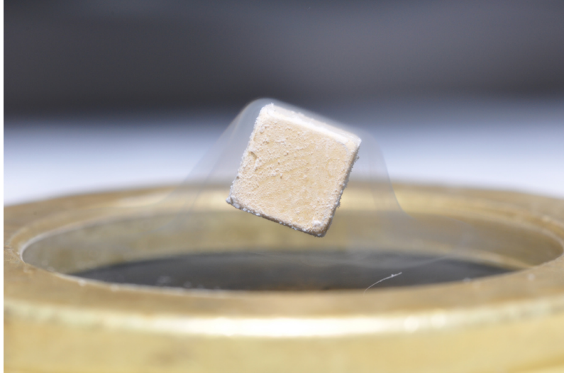
Figure 3. Demonstration of the Meissner effect of type II superconduction. Superconductor is levitating on top of a magnet. Photo by Mike Bell https://www.flickr.com/photos/mikedbell/4131403101/
