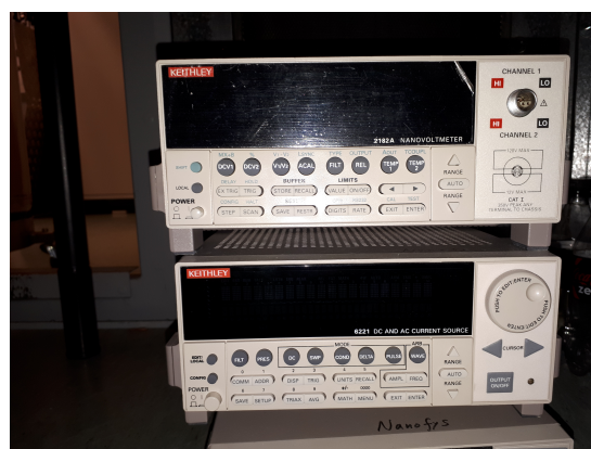
Figure 27. Above Keithley 6221 dc and ac current source and below Keithley 2182A nanovoltmeter.
