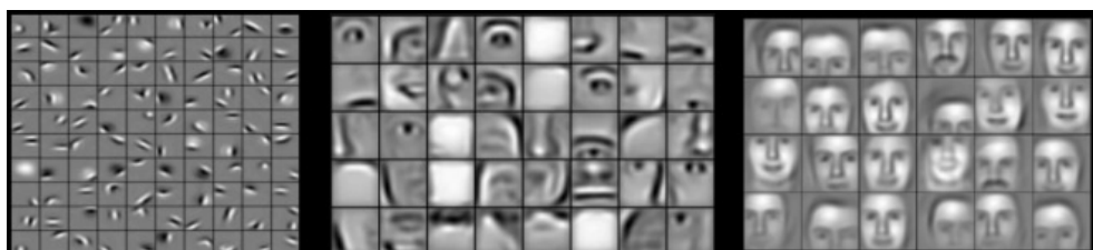
Figure 12: Example of kernels learned by a 3-layer CNN (Lee et al. 2009)
