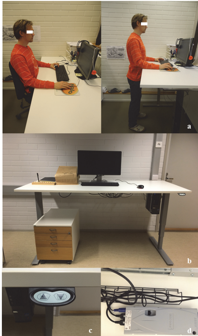
FIGURE 3 Electronically adjustable sit-stand workstation (ISKU, Finland). The participant used a sit-stand workstation for office work (a). The workstation was adjusted for standing work at a height of 100 cm (b). Adjustment panel with two buttons for height adjustments (c). Electrical engine system and storage basket for wires (d).
