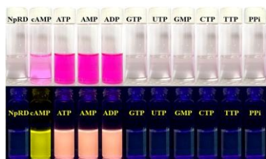
Fig. 3. Photograph of visual (upper panel) and fluorescence (lower panel) color changes of NpRD ( c = 2 \times 10^{-5} M) in \text{CH}_3\text{CN}/\text{H}_2\text{O} (1:6, v/v) (pH 7.0) after the independent addition of 6 equivalents of various nucleotides and biological phosphates in 10^{-4} M concentration.
