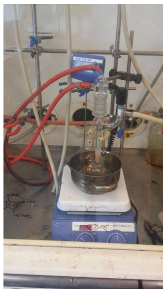
Figure 26. Examples of a) sublimation with a sublimation apparatus and b) combined degassing and reduction with an H-cell.
