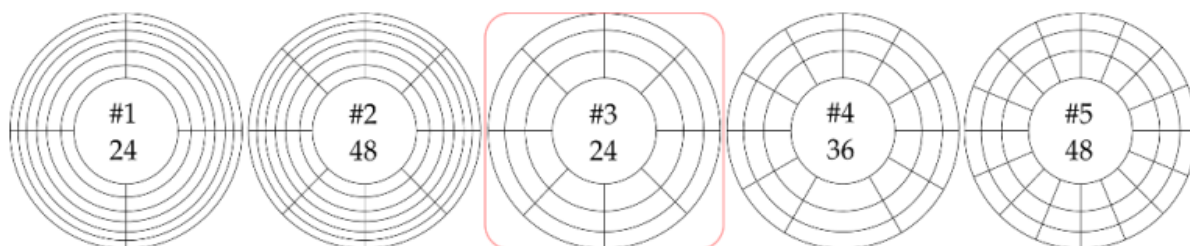
Figure 17: Different silicon detector designs for SPEDE. Figure taken from [33].
