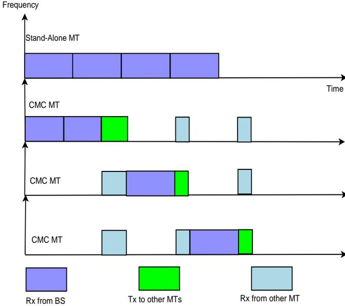
Figure 2. Transmission procedure
