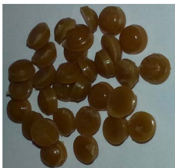
Fig. 3a) PVC (NMIJ 8123-a) pellets before autoclave digestion method A 3b) PVC pellets after the digestion method A
