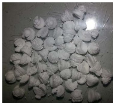
Fig. 3a) PVC (NMIJ 8123-a) pellets before autoclave digestion method A 3b) PVC pellets after the digestion method A
