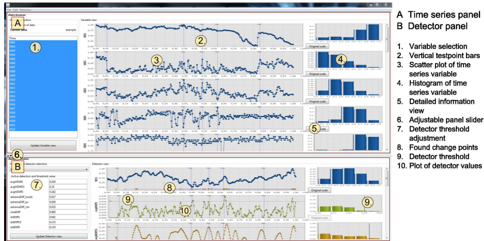
Figure 2. Java GUI with example data. In the upper panel, time-series data is visualized. Change points are analyzed on the lower panel.
