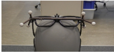
Figure 2. The tracking system used in the wave field synthesis condition on the dummy head.
