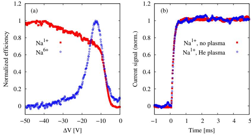
FIG. 1. (a) Normalized breeding efficiencies of  $^{23}\text{Na}^{1+}$  and  $^{23}\text{Na}^{6+}$  as a function of  $\Delta V$ . (b) Time-resolved Faraday cup signals of  $^{23}\text{Na}^{1+}$  with and without helium plasma in the charge breeder ( $\Delta V = -12.9$  V).
