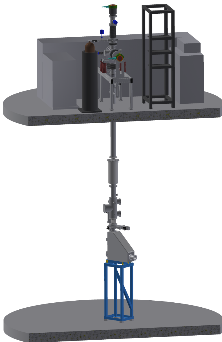
Figure 13: The newly commissioned vertical beam line
