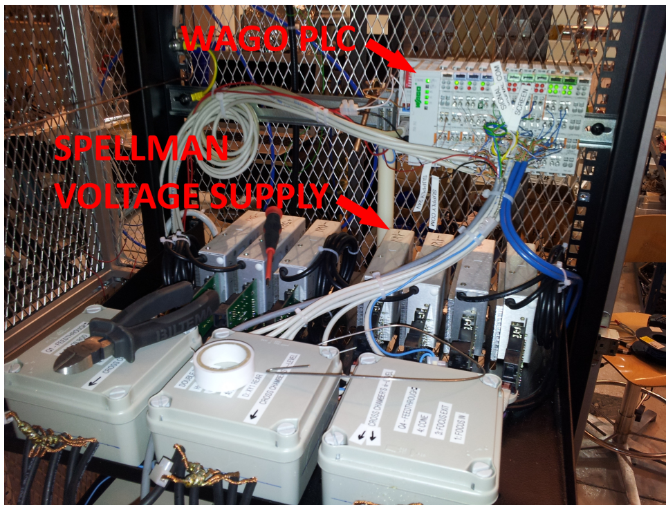
Figure 26: a PLC and a part power sources of the off-line set-up
