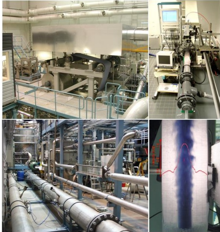
Figure 11: Examples of industry-related research facilities at VTT. Part of the paper machine short circulation research environment 'SORTTERI' (upper left). Optical tomograph device developed by University of Jyväskylä during tests at VTT (upper right). Pilot scale flow facility at VTT (lower left). Velocity profile in mixing flows measured using ultrasound Doppler method (lower right).
