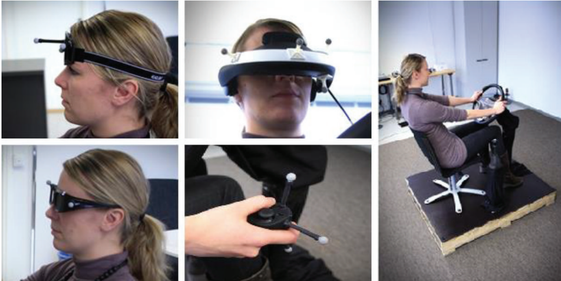
FIGURE 1: The devices used in the experiment: upper left: headband; lower left: 3D glasses; upper centre: head-mounted display (HMD); lower centre: the controller; right: car skeleton.
