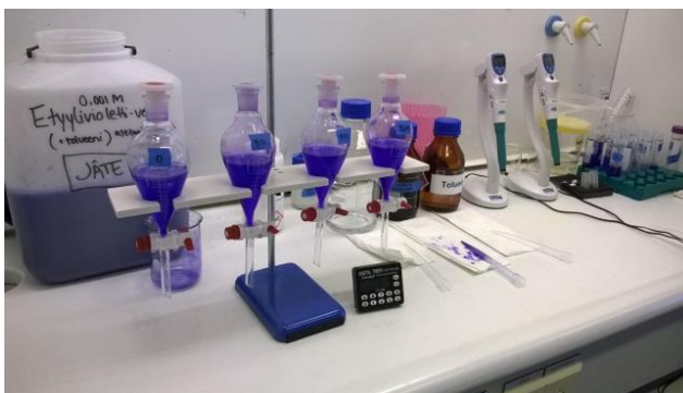
Figure 29. SDS-analysis and toluene extraction: layers of water and toluene are let to separate for 30 minutes
