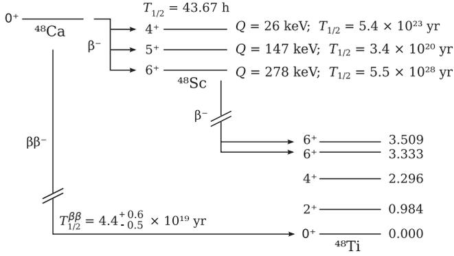
FIG. 1.  $\beta$ -decay scheme of  $^{48}\text{Ca}$ . In addition to the three ordinary  $\beta$ -decay branches of  $^{48}\text{Ca}$ , the ground-state-to-ground-state double- $\beta$ -decay branch  $0^+ \rightarrow 0^+$  is also shown. The values for the partial half-lives of the ordinary  $\beta$ -decay branches are taken from Table I with  $g_A = 1.25$ . For  $^{48}\text{Sc}$ , only the dominant decay branches are indicated.
