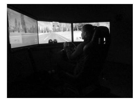
Figure 4. The motion-base medium-fidelity driving simulator
