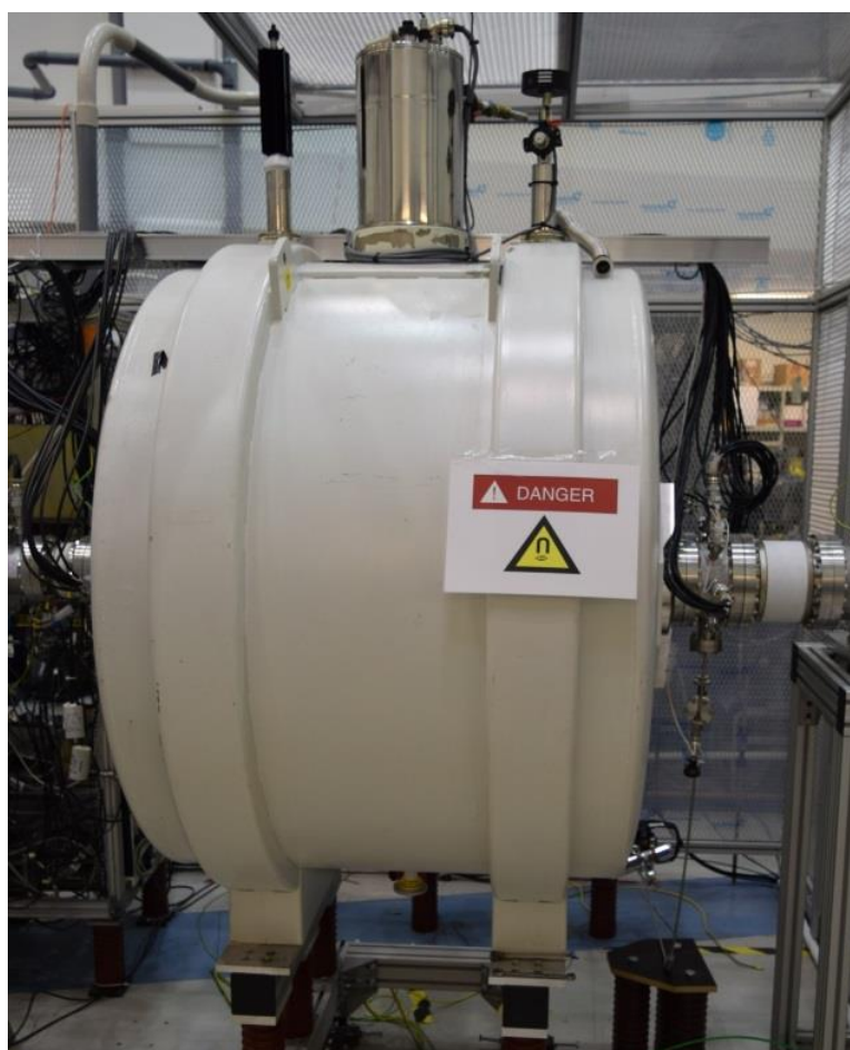
Fig. 2.5: The superconducting solenoid of the JYFLTRAP Penning trap.
