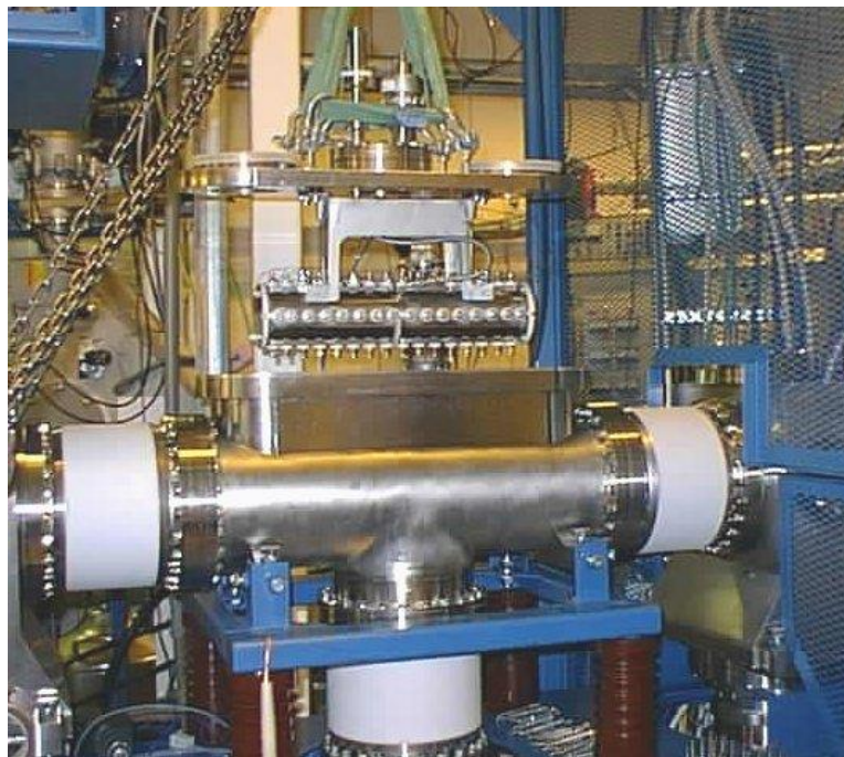
Fig. 2.4: The RFQ structure taken out from the vacuum chamber.
