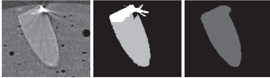
(a) Original data with star artefact. (b) VaWe filtered and segmented. (c) Gaussian filtered and segmented.
