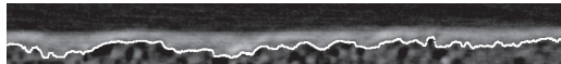
FIGURE 61 Bottom surface of a coating layer of paper. This surface is shown as a thick white line beneath the coating.
