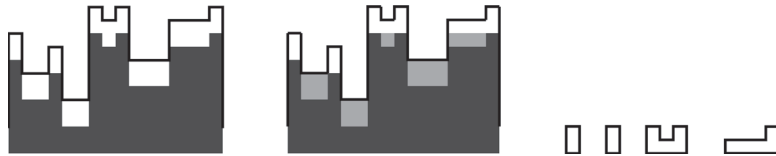
FIGURE 35 A 2D example of the geodesic reconstruction. On the left the black line represents the original image, and the gray area is the G . In the middle the algorithm 2 has been applied to G ; the lighter gray areas are filled by the reconstruction. And on the right is the difference between the original and reconstructed G .
