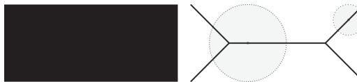
FIGURE 34 A square object (on left) and its skeleton (dark line) with few maximum balls shown.
