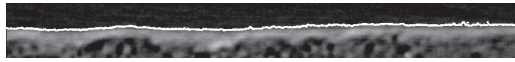
FIGURE 60 Top surface of a coating layer of paper. This surface is shown as a thick white line above the coating.
