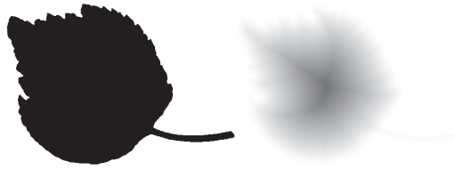
FIGURE 33 A binary image of a leaf (on the left) and its distance transform (on the right). The darker colors depict longer distances.
