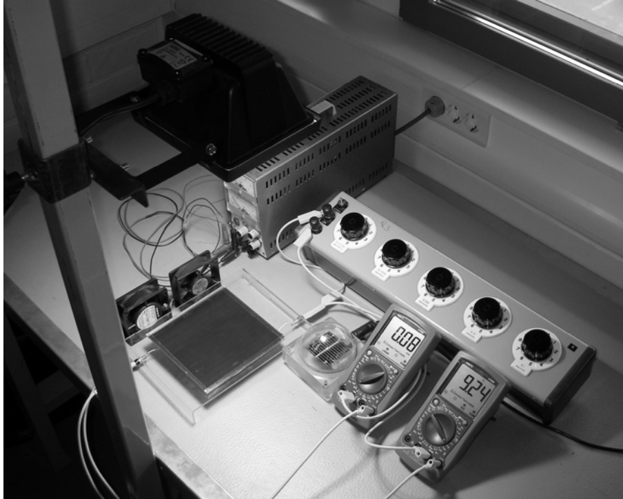
Figure 3. Photograph of the experimental setup. The square 15 x 15 cm 2 PV cell is illuminated using a standard halogen lamp whose height (and irradiance) can be adjusted by means of a vertical steel support. Cooling fans can be seen to the left of the module. Resistance values can be dialled into the decade resistor, shown on the right.
