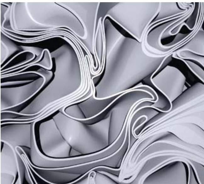
Fig. 1. Internal structure of a crumpled elasto-plastic membrane
