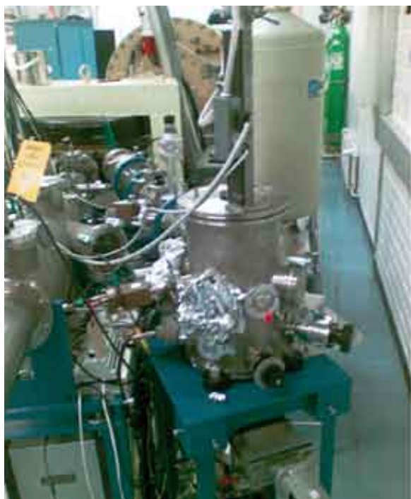
Fig. 3. Beam line and end-station for PIXE/RBS analysis.
