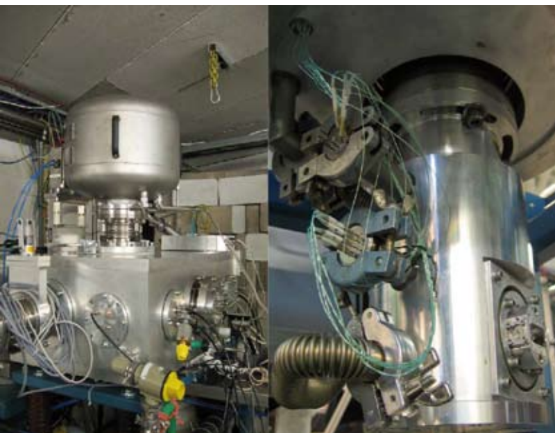
Fig. 2. Cryogenic ion guide. Left: liquid nitrogen dewar mounted on top of the IGISOL vacuum chamber. The primary beam enters from the left. Right: view of the ion guide mounted on the end of a cold finger, surrounded by heat shielding which is also under vacuum.
