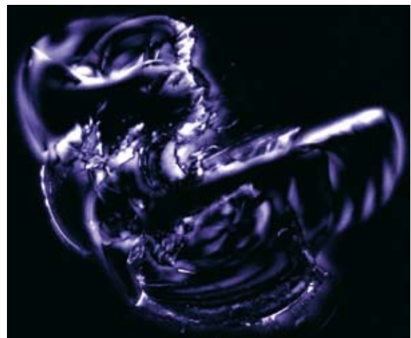
Fig. 1. Microfractures in a sapphire crystal.
