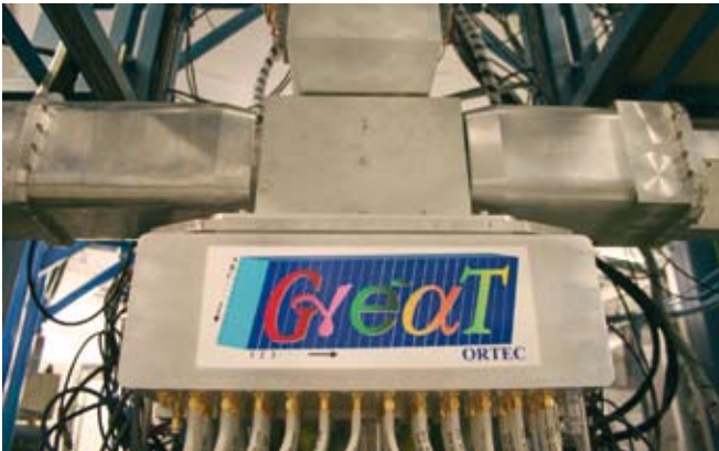
Fig. 2. Two GSI large-volume Clover germanium detectors installed with the GREAT spectrometer.
