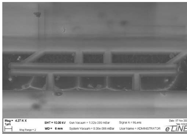
Fig. 2. A suspended mesoscopic AlN structure.
