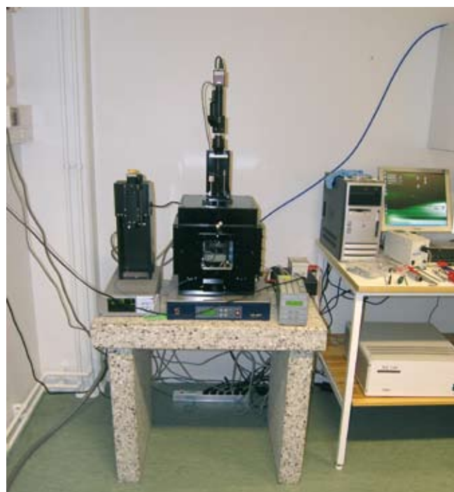
Fig. 17. A commercial AFM (PSIA XE-100) placed inside an environmental chamber.
