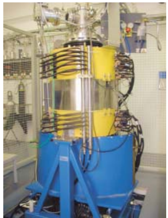
Fig. 2. The upgraded 6.4 GHz ECR ion source.
