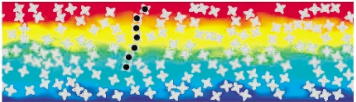
Fig. 9. A snapshot of a shear flow of star-shaped particles suspended in a fluid. Red color indicates high fluid velocity. A typical example of cluster is also shown in the figure
