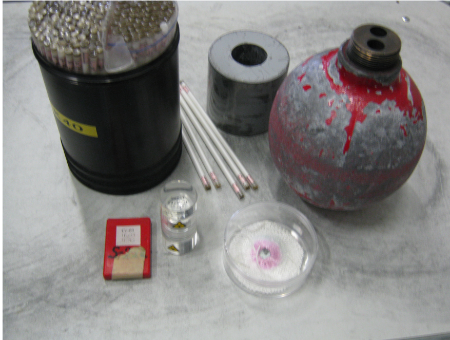
Figure 20: Equipment used in the measurements: ^{40}\text{K} rods, collimators, 370 kBq ^{60}\text{Co} source, 2582.6 Bq ^{241}\text{Am} source and gas mantle containing thorium and other radioactive materials from its decay chain.
