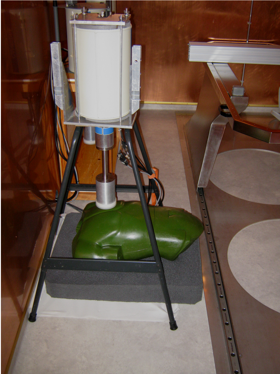
Figure 13: Photo of the measurements with the phantom in the low background chamber.
